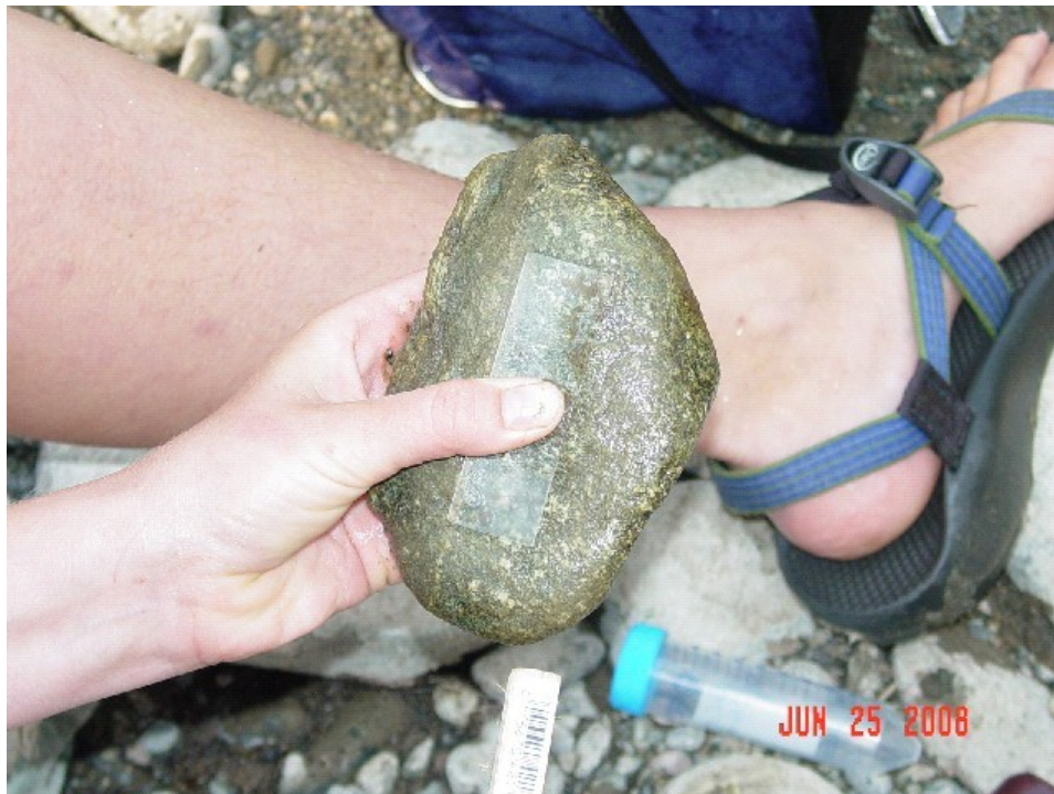
Figure 10. Sample area equivalent to a 1" X 3" microscope slide is selected prior to scraping. Photo was taken by KTWQP staff at Klamath River Orleans site in June 2006.
