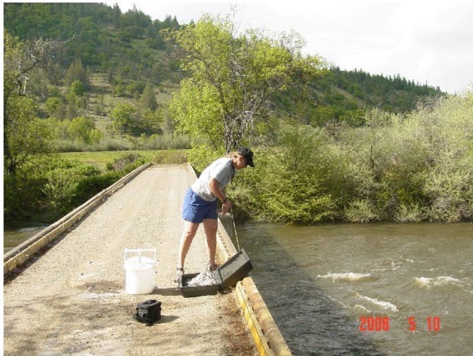
Figure 8. KTWQP staff collects Klamath River water using a Van dorn sampler and then deposits in churn to ensure representativeness of sample. Photo taken in 2006 at Klamath River above Copco Reservoir.
